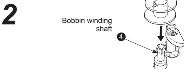
● Set the bobbin on the bobbin winding shaft ④.
